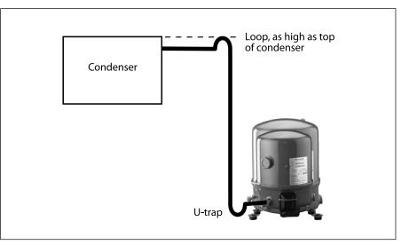
In most installations the initial compressor oil charge will be sufficient. In installations with line runs exceeding 20 m, or with many oil traps, or an oil separator, additional oil may be required. In instal-
