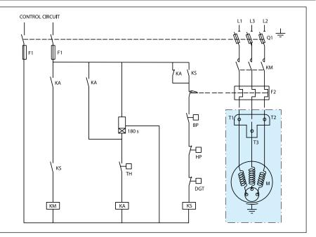
Starting current of Maneurop® 3-phase compressors can be reduced by using a soft starter. Two different versions are available: CI-tronic<sup>™</sup> soft starters type MCI (recommended) and soft start kits with statoric resistors (type SCR). Starting current can be reduced by up to 50% depending on the compressor model and the type of soft starter. Also mechanical stresses that occur at starting are reduced, which increases the life of internal components.
