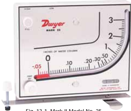
Fig. 13-1, Mark II Model No. 25 inclined-vertical manometer. (shown with optional A-612 portable stand)
